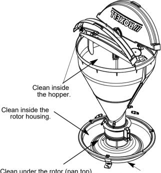
Clean under the rotor (pan top) Clean under the pan.
